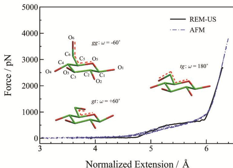
**Figure 1.** Comparison of force spectra obtained from the REM-US simulations (black solid line) and AFM experiments (blue dash-dot lines). Three major conformations involved in the stretching process are shown in the plot, corresponding to the rotamers: gauche-gauche (gg), with the dihedral angle O6-C6-C5-O5 (denoted by the red dash lines in the molecules)  $\omega = -60^\circ$ ; gauche-trans (gt), with  $\omega = +60^\circ$ ; and trans-gauche (tg), with  $\omega = 180^\circ$ .
